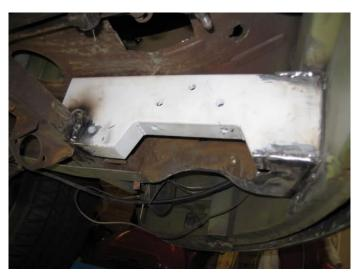
7. The rear section can be welded, accessed through the Brake Reservoir panel in the floorpan
