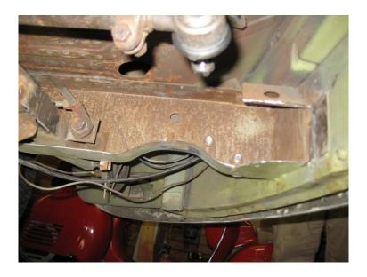
5. Position the brace against the inner valance and main chassis rail. Note the area on the main chassis which has been relieved to allow the steering box to be raised
