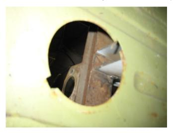
8. Clearancing the floorpan to allow the steering box pitman arm to rotate without obstruction
