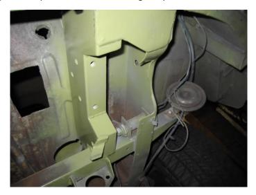
9. Test refit the steering, and brakes. With the wheels and steering centred, you will find the pitman arm needs shortening approx 10mm to align as before. Fabricate a small fillet to the floorpan. The section of metal further back will also need releiving to clear the drag link
