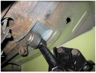
10. Notch and reinforce the brake pedal arm as necessary to clear the steering box.
