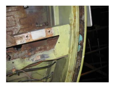
4. Remove the original chassis section, grinding clean the front inner valance areas and rear cross member box section.
