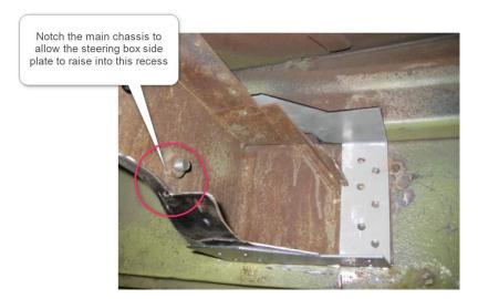
6. Offer up the main section and weld in place
